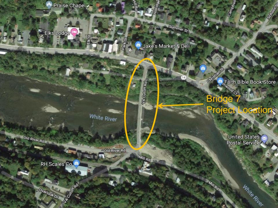
Looking North over Bridge **Existing Conditions – Bridge #7** Roadway Classification – Local Road (Class 2 TH) Bridge Type – 559' Long 4-Span Steel Deck Truss Ownership - Town of Hartford Constructed in 1929, Reconstructed in 1973
